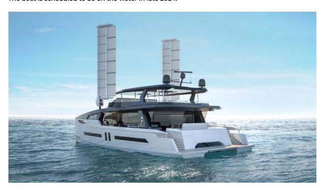
The Oceanwings® system of AYRO has been refined through data collected from use on Energy Observer, which has sailed more than 50,000 nm with zero emission. The operating principles of the Oceanwings® are comparable to an aircraft wing turned upright that provides horizontal 'lift' (instead of vertical) to propel a boat. They are automated, with sophisticated software that monitors and analyzes wind and water conditions, and adjusts the angle of attack of the wingsail for optimum efficiency.
